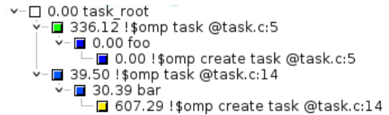
Figure 9: Explicit tasks call path in the task granularity test program (shown metric is the execution time).
