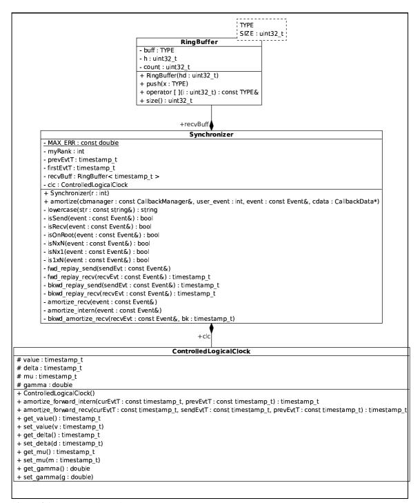
Figure 4.1: Program Class Diagram.
